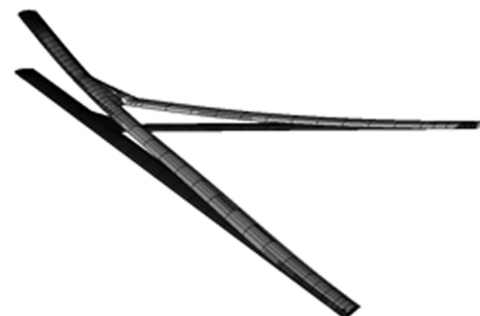
Fig. 17 Deformation from nonlinear analysis of the optimum design using ELs.
